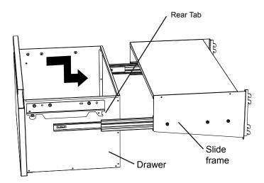
2. Pull out slide arms and drop rear tabs on drawer into slots on the slide arms. Rotate down and push drawer in. (Do not install Set Screws)
