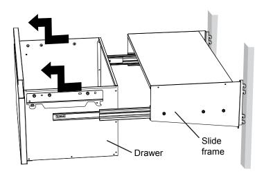
**4.** Once drawer has been set in proper location. remove drawer leaving the top support in place.
