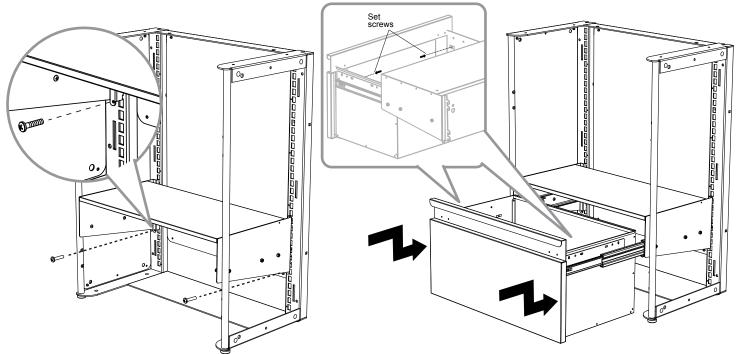
**5.** Install (2) securing screws.
