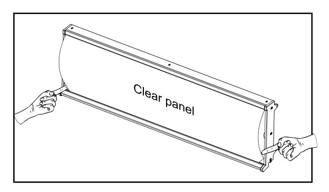
**5.** To install or replace graphic, lift and remove clear panel from corners as shown. Remove protective film from clear panel. Place graphic, and reinstall panel. When header has multiple graphics required, install graphic and apply vinyl strips **(D)** to plastic cover over graphic seam. Use narrowest vinyl strip possible.
