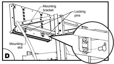
**3.** Secure the light fixture onto the metal fixture by pushing the locking pins (2) through the holes in the mounting tabs and into the mounting bracket. Do this on both mounting brackets (Fig. D). Route power cord and secure with supplied cable ties and cord clips (see "Power Cord Routing" installation sheet).
