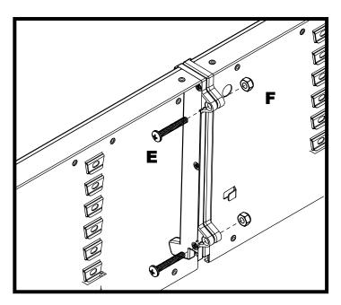
**4.** With multiple header assemblies, secure adjacent sign frames using 2x #10-24 Phil Pan Head **(E)** and 2x #10-24 Lock Nut **(F)**.
