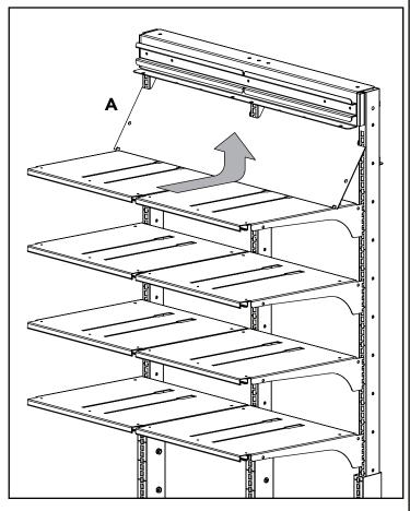
2. Secure Shelf Blocker (A) using 3x Push Fasteners (B).
