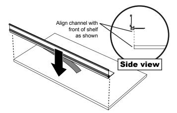
1. Remove adhesive backing and adhere front channel to clean shelf surface. Ensure channel aligns with front of shelf as shown (see side view).
