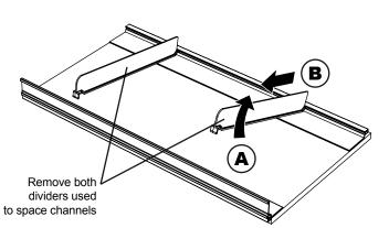
**3.** Remove dividers by pulling up on front (**A**) and pulling forward to disengage rear (**B**).
