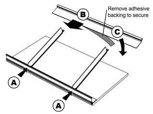
IMPORTANT: To space rear channel from front channel, temporarily insert (2) dividers into front channel (A). Insert rear of dividers into rear channel (B). Lift rear channel, remove adhesive backing and lower to secure to shelf surface (C).
