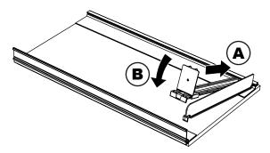
Install dividers and pushers as shown. Push in back of each element (A), then rotate down into front channel (B). To ensure proper spacing of pushers and dividers, insert product to be merchandised into pusher track, then install adjacent divider and pusher.
